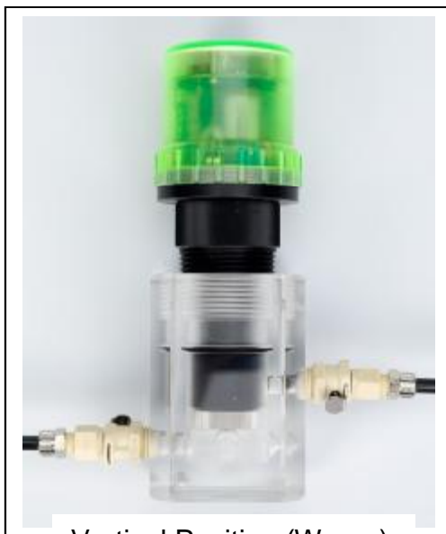
Vertical Position (Wrong)
