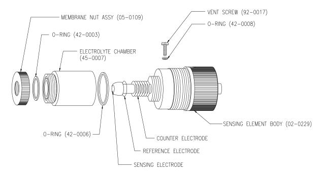
Figure 2 - Cl2 Sensor Assembly
