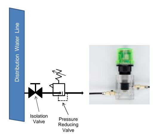
Figure 1 - Typical ChlorLog Monitoring Installation
