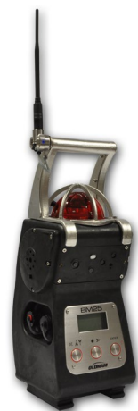
Figure 20 : Wireless version, recognizable by the presence of an antenna
